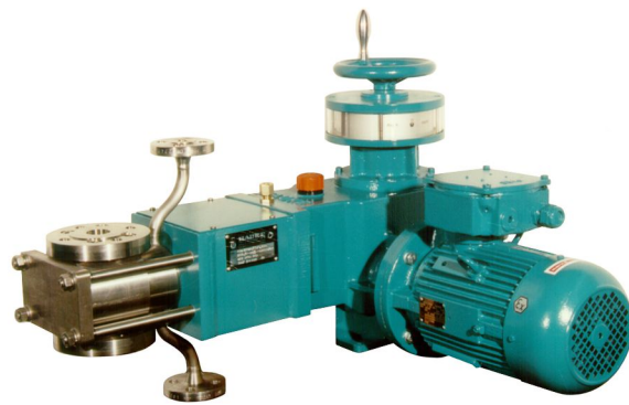
PIM K plunger-metering-pump with stroke adjustment by hand-wheel and with stuffing box and lantern ring
